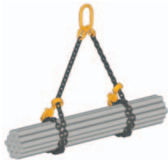
2-legged wrap and choke hitch.
